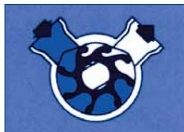
When the flexible vanes again contact the eccentric cam they bend with a squeezing action which provides a continuous, uniform discharge of liquid.
