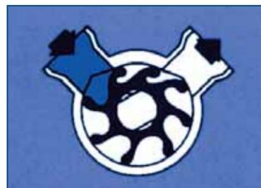
Flexible vanes create increased volume when leaving the eccentric cam creating a vacuum thus drawing in liquid, instantly priming the pump.
