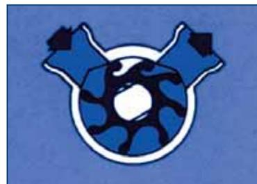
As the flexible vanes rotate, the liquid is carried through the vanes from the inlet to outlet port, each successive vane drawing in liquid.
